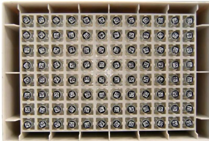
Figure 1 – Bottom view of specimen tray containing 96 test tubes.
