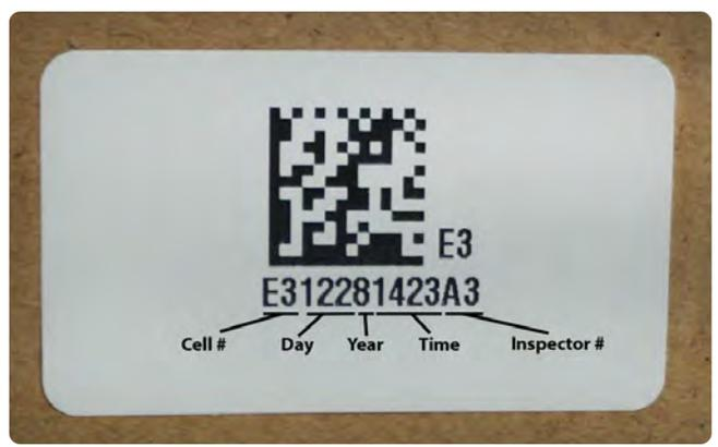
**Technology:** This particular set-up involves a Zebra printer (ZD500) along with an Ultra-Rugged Zebra bar code scanner (3600 series). However, this solution is scalable on any Zebra printer that utilizes the Link OS. The custom program written by the EMP software engineers is what ties the inputs from the bar code scanner to the printer itself.
