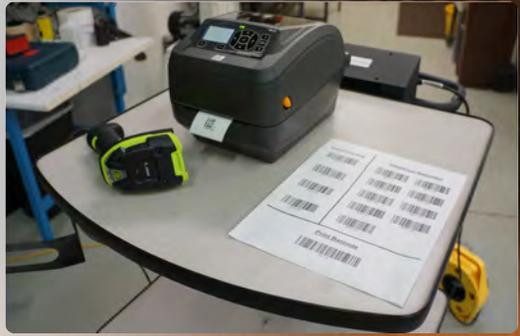
EMP Technical Group's team of engineers designed a clean, simple, and cost-effective solution. By utilizing Zebra Basic Interpreter (ZBI), the software engineers at EMP were able to write a custom program that allows the bar code scanner to connect directly to the printer. This eliminates the need for a PC!
