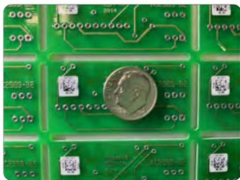
The process was difficult to automate as the size of the panel could be as large as 16" x 10", have as many as 96 barcodes and contain barcodes as small as 1/4" x 1/4". The panel configurations also change frequently throughout the day. The EMP engineers knew they wouldn't be able to use a fixed mount barcode reader. Instead, they designed a solution utilizing a line scan camera integrated with a conveyor.
