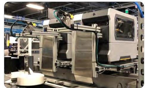
In order to further enhance the throughput of the system, EMP installed two of the ZT620s side-by-side so they could simultaneously fill two separate boxes. This solution has dramatically reduced the amount of downtime while at the same time greatly improving the overall accuracy of the process.
