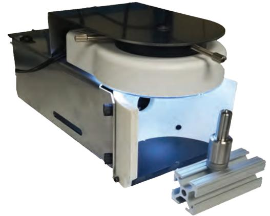
Unfortunately, the customer was experiencing significant downtime on a number of the barcode scanning lines. As the part comes into view of the Cognex Dataman, a vision light is triggered to illuminate the DataMatrix code. Instead of highlighting the 2D code, the vision light was creating a bright hotspot right on top of the code itself. This caused many no-reads by the Dataman.
