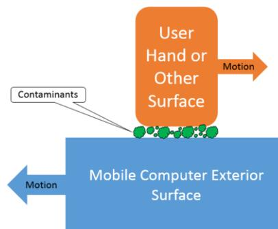
**Figure 1: Three-Body Abrasion**
