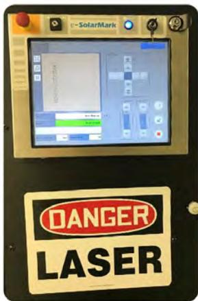
For the container, the customer installed a robot to pull the container out of the mold and placing it on a conveyor. The EMP engineering team then designed a fixture to position a Matthews e-SolarMark Co2 laser over the top of the conveyor and to mark the part with an exact time and date as it passes by. The date/time stamp is critical; therefore, EMP decided to include a Cognex InSight 2000 with custom lighting that verifies each mark has been made.
