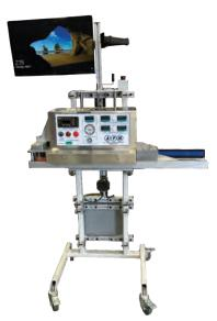
The team at EMP designed a solution using Cognex's InSight 7802, 5MP camera. This would allow them to read the barcode and complete the character recognition in one device. The EMP team also created a custom mount so the camera can mount directly to the sealer.
