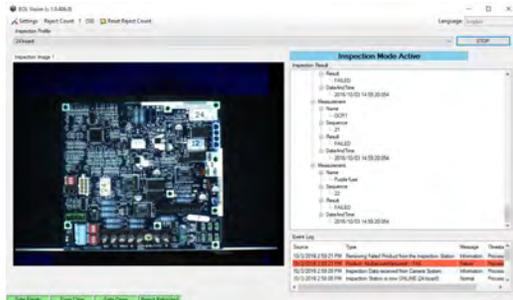
Because of the circuit board variety, the team at EMP knew right away that a custom program that would allow the user to select which board they were running would be needed. This program is visually displayed on an HMI that is powered by a Windows PC. It allows the user to select the job they want to run as well as program any new jobs that may arise.
