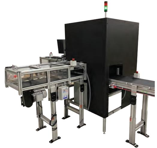
This is a complex application, but the vision engineers at EMP were up to the task. Each circuit board is placed on a conveyor and sent through to the vision inspection. A 12 MegaPixel GigE color camera, along with the vision software, performs a number of inspections to identify each manually placed component:
