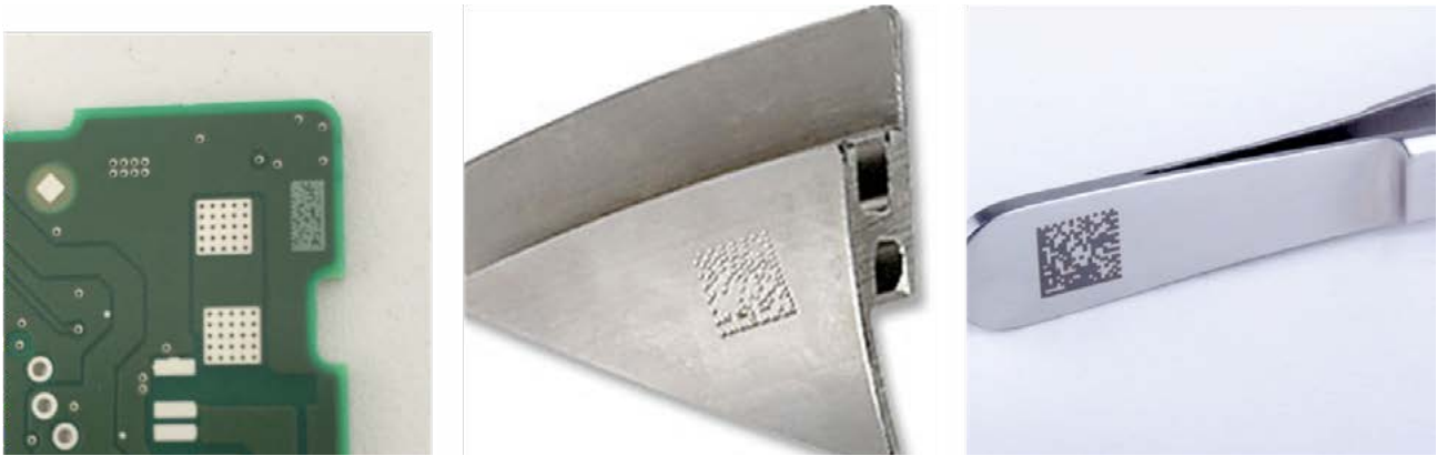
Figure 2. Direct part mark (DPM) codes are commonly used in many industries which mandate verification.
