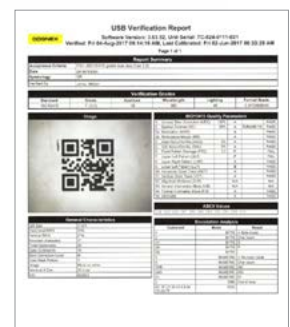
Figure 4. Barcode readers are designed to reveal and read the data within a code. Some barcode reader software may provide print quality metrics useful for process control. Barcode verifiers, by contrast, grade codes according to international standards and generate printed reports to help demonstrate compliance.
