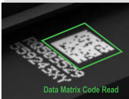
Figure 4. Barcode readers are designed to reveal and read the data within a code. Some barcode reader software may provide print quality metrics useful for process control. Barcode verifiers, by contrast, grade codes according to international standards and generate printed reports to help demonstrate compliance.
