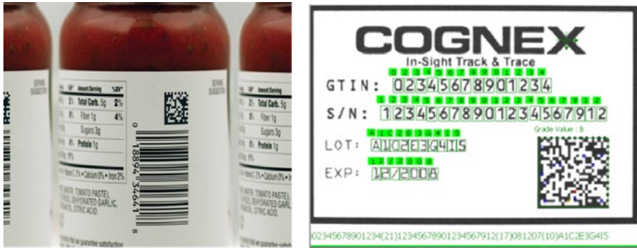
Figure 6. Identification techniques can range from simple barcode scanning to OCR.
