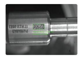
When a noread signal is sent, the Dataman continues to trigger in hopes of getting a good read. As the Dataman triggers over and over, the production line waits until an operator is able to come over and manually rotate the part to try and remove the hotspot.
