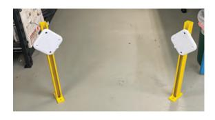
driver approaches the destacker with their given orders, the pallet jack is scanned. The jack then removes two pallets. Each pallet is also scanned as the pallet jack exits past the RFID antennas. The operator proceeds to fulfill the customer order and the order is tied to the specific pallets that were scanned.
