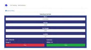
After assessing the situation, EMP knew right away that this would require a custom program to store all the information. The solution that EMP provided involved an ultra-rugged Zebra handheld barcode scanner that scans the initial tag's barcode to obtain any information available. Any missing data is manually entered in the program on a PC. Next the coil is weighed and verified against the weight given by the vendor. Any discrepancies are taken up with the vendor. Once the information is
