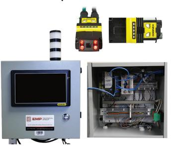
Stationary Matchcode involves similar logic, but in a stationary setting. The items are able to move down an assembly line while simultaneously being read against the control barcode to ensure there's a match. This particular setup is administered by a custom EMP built PLC.
