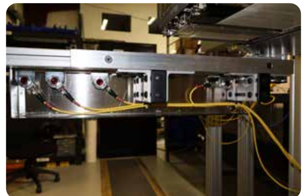
Sensors for identifying presence and correct size part
