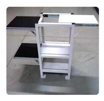
a custom design solution. By using 80/20, they were able to build and then bolt on shelves to the back of the stand allowing for perfect placement for label storage. Now they can load the fan labels, and essentially walk away as thousands of labels are printed.
