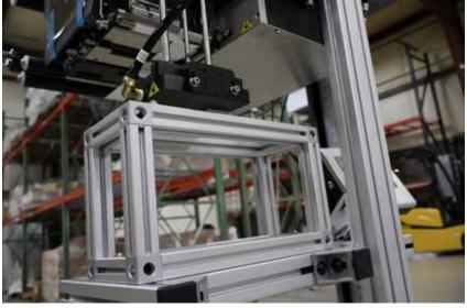
They built a cradled tower with interchangeable custom 3D-printed plastic fixtures for different part boxes and attached a pedal trigger for on demand labeling. Operators can easily switch fixtures, adjust settings on the display interface, and press the pedal to label efficiently. This solution resulted in a faster, error-free workflow.
